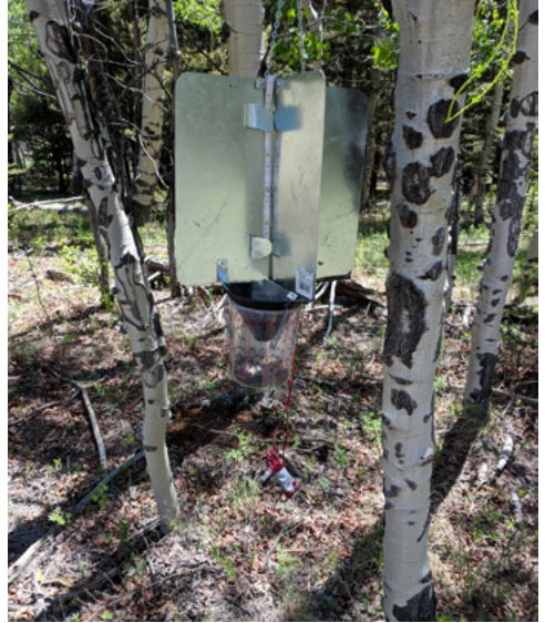
Figure 2. A moth trap used to sample moths across the study area. LED lights attract moths to the trap where they are captured for subsequent identification, counting and calorimetry.
